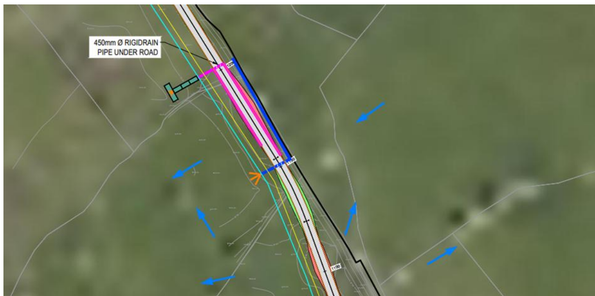
Figure 5-1: Typical drainage design
